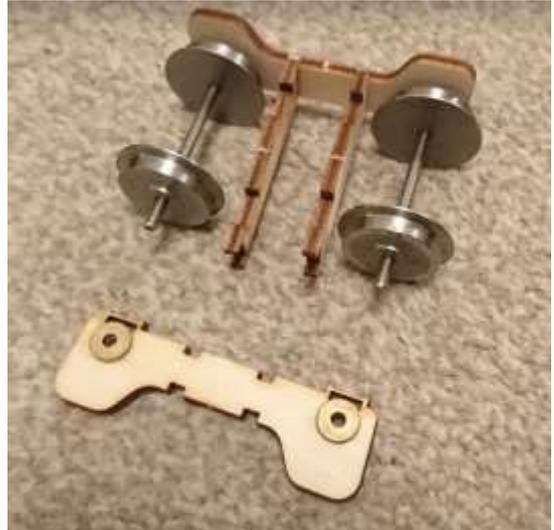
Glue the top crossbar piece with the pivot hole in place. This will lock the bogie frame in square.
