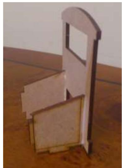
Locate the cab back over the battery box onto the loco floor
