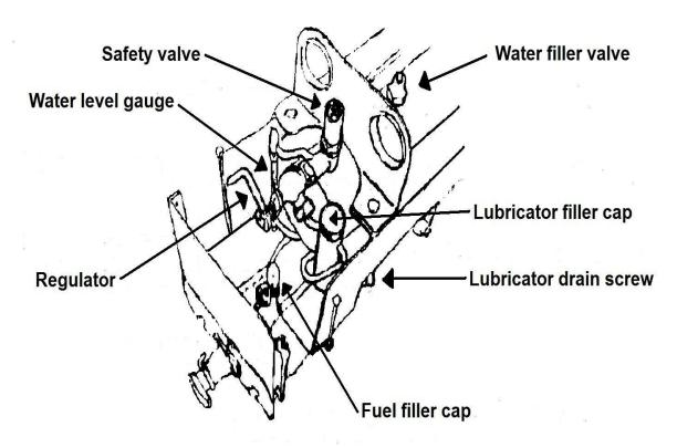
Soft water must be used in the boiler; generally tap water is hard and not suitable. Distilled water used for steam irons or battery top ups is commercially available and suitable. To fill the boiler either unscrew the safety valve and fill, or use the small syringe supplied and the water filler valve. To do this fill the syringe with water insert the nozzle squarely on to the filler valve located on the boiler top and squeeze the syringe – do not apply unnecessary force to the locomotive.
