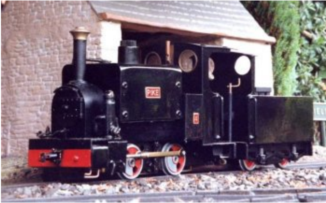
Another of my modified Mamods fitted with a displacement lubricator, meths fire with fuel tank in the tender, cylinder covers, boiler vacuum filler drawing water from the tender, cab control lever etc.
