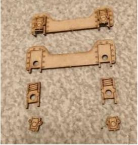
Glue the overlays in place on the bogie sides, being careful not to allow glue to contaminate the axles or bearings.
