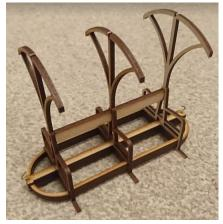
Glue the second end frame in place. Then apply glue to the centre frame.
