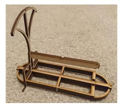
Glue the backrest into one of the end frames. Make sure that the centre notch in the backrest is placed to the top
