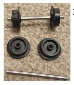
Assemble the wheel sets to suite your gauge. The wheels are friction fit. No gluing required.
