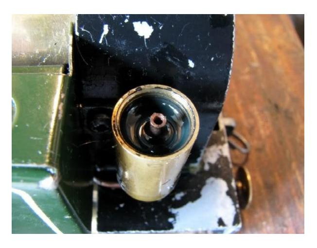
I have also successfully fitted a Dream Steam Lubricator into the New Mamod Locomotive Mark 1.
