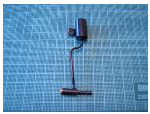
It needs to be bent again just at the bottom of the first bend, so that it will go through the cut out in the chassis frame at the front of the combustion chamber, and then further bent to align the T piece with the steam in port on the regulator/reverser valve.
