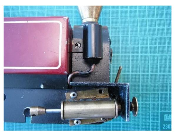
The T piece portion of the lubricator can foul the cylinder pivot screw and the regulator/reverser valve pivot screw as well.
